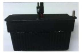
The battery has one plug with two connectors (+) and (-). It is constructed that it can be plugged into the mating connector one way.
