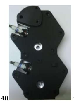
Thermostat located outside dewatering plate.
