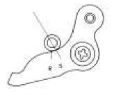
Turn the handle grip so that the collar center of the carburetor throttle lever in on the "S" marking line.
