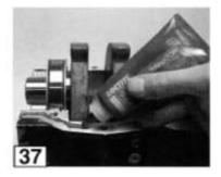
**38 39** 11. Head gasket requires adhesive. Recommended is Permatex Aviation cement. Install head gasket to Raider 40 outboard. Gasket is required between head and dewatering cover plate. Permatex Aviation cement is recommended. This gasket material does not harden like typical cement; excellent for submersion characteristics.
