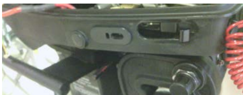
Slide Lever to rear –opens valves
