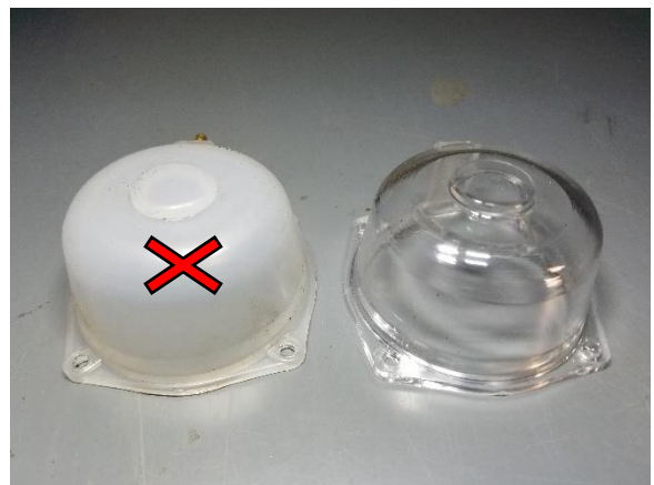
Fig (2) 40 HP Carburetor Bowl, , red X indicated improper part
