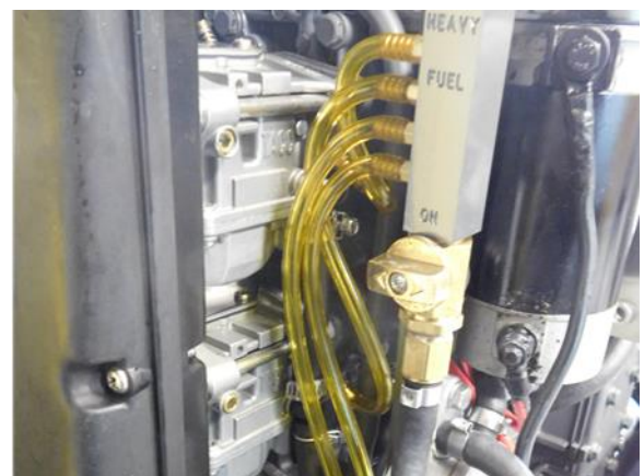
Fig (10) Raider 50HP with Tygon tubing fuel line
