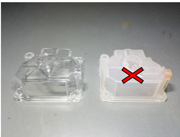
Fig (1) 50HP Carburetor Bowl, red X indicated improper part
