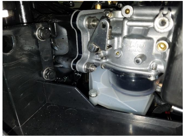
Fig (4) 40HP Carburetor Bowl, installed
