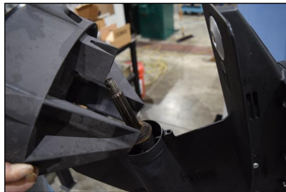
Img 2b. Install stator
