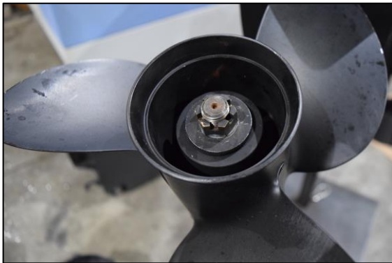
Img 1a. Cotter pin removed
